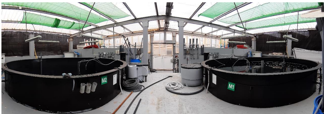
Figure 1.6. Larval rearing in Mesocosms tanks (40 m 3 ) for research purposes (ECO-AQUA facility, ULPGC, Spain).
