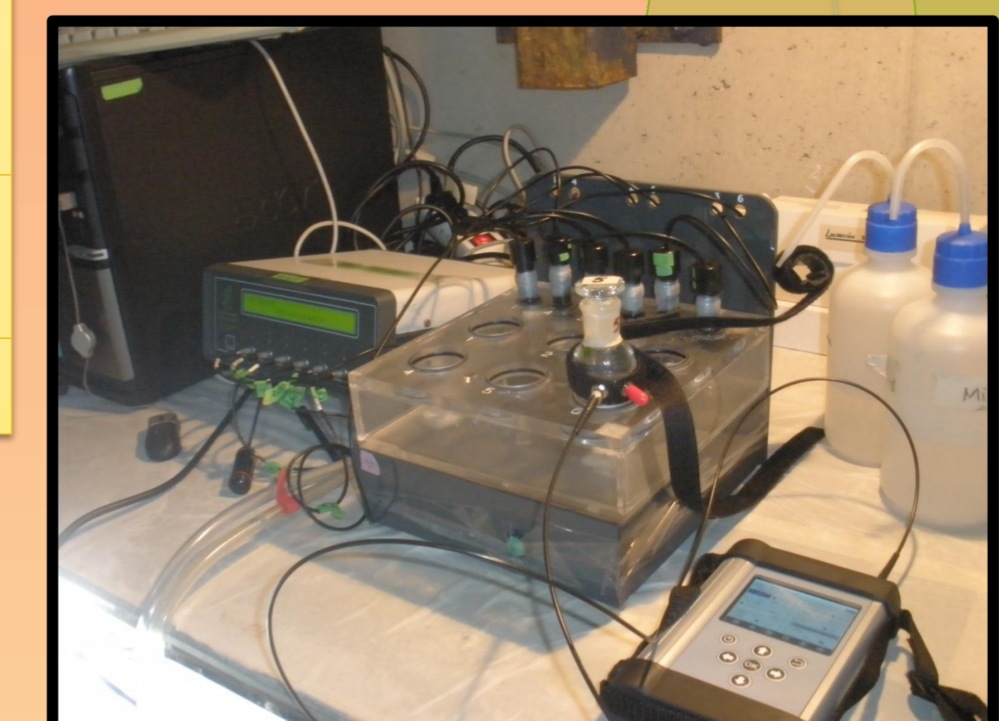
Figure 4. We are studying respiration using optodes (Fibox 4, Presens) in order to describe the impact of light and darkness on metabolism.
