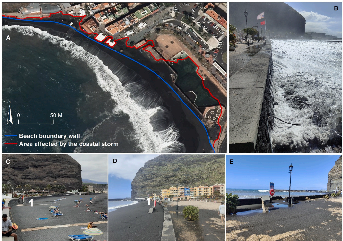
Fig. 11. Effects of coastal storms on Tazacorte beach and seafront. A) Orthophoto of 2021 showing the area affected by storm Kamiel (source: IDE Canarias. GRAFCAN S.A.). Photos of the effects of storm Kamiel (3rd of March 2023): B) The seafront at Tazacorte beach being affected by waves; C) Access walkways at the backshore before the storm; D) Buried access walkways and sand on the seafront; E) Sand on the beach seafront.
