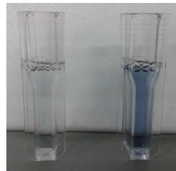
Fig. 10. Examples of cuvettes for protein measurement of different protein concentration during Lowry's method.
