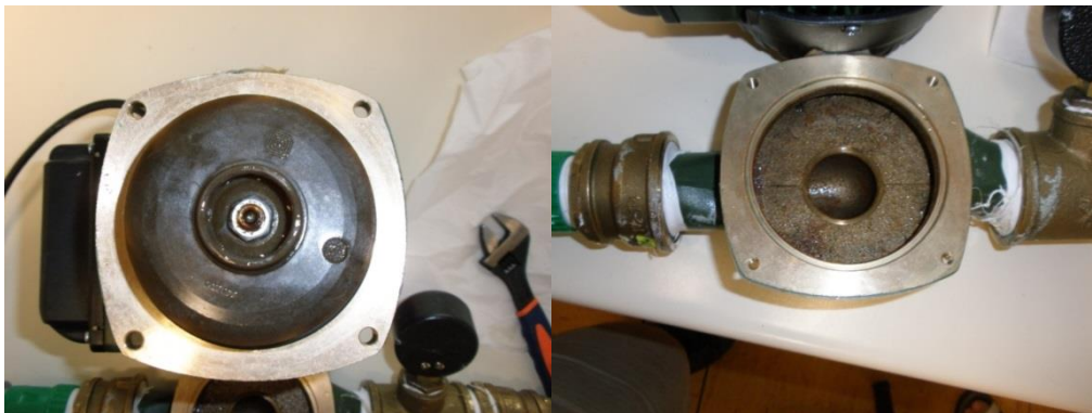
Figure 3-13: Photos of the pump ALP 800. Impeller mounted on the rotor (left). Volute, inlet and outlet pump (right).
