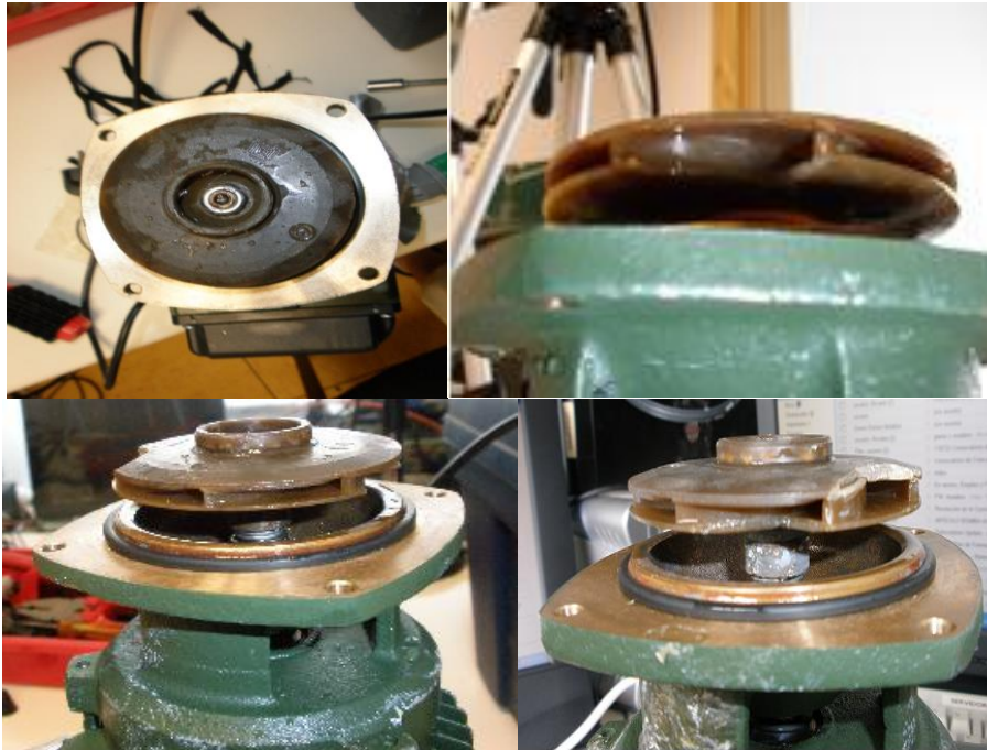
Figure 3-15: Photos of the plate fault in impeller. Upper left: impeller in normal condition. Upper right: one part of the plate removed. Lower left: two parts of the plate are removed. Lower right: the third part of the impeller was removed.
