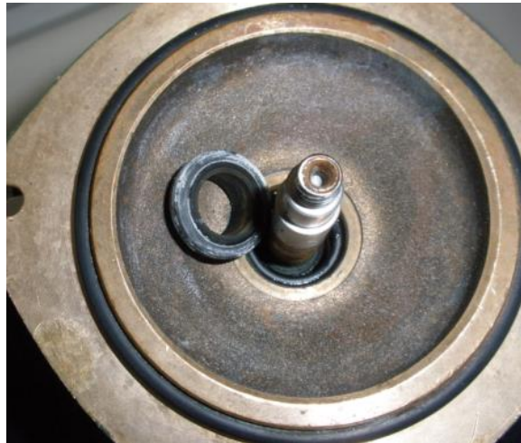
Figure 3-18: Photo of the o-ring of the impeller of the AL P800 pump.
