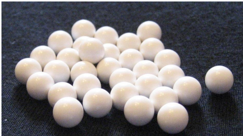
Figure 3-20: Kind of PVC balls (6 mm of diameter) used to simulate strange objects in the system [29].
