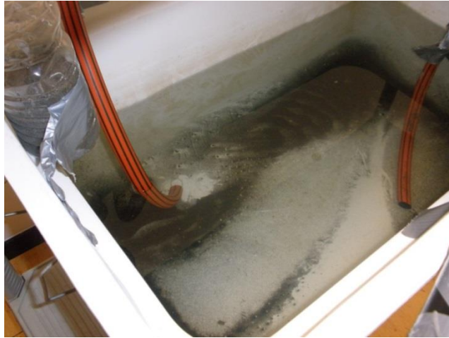
Figure 3-19: Photo of the reservoir with the sand added to simulate strange objects or particles in the system.
