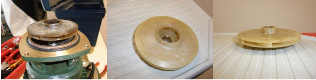
Figure 3-14: Photos of the pump ALP 800. Impeller mounted on the rotor (left). Different views of the impeller (center and right).
