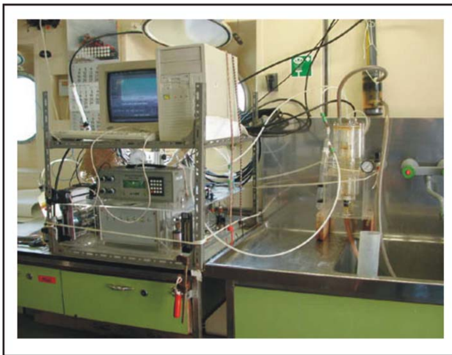
Figure 13.- Equipment for continuous underway pCO 2 measurements
