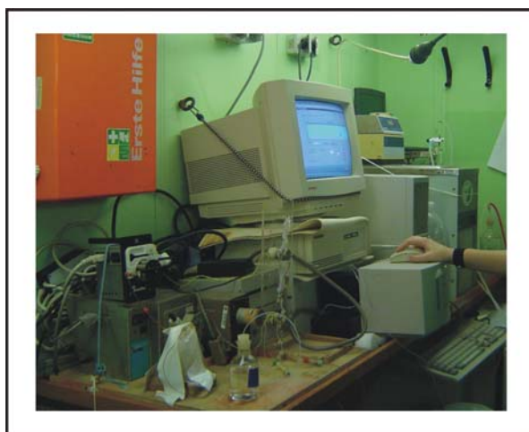
Figure 9.- pH analysing system set up for on board analysis.
