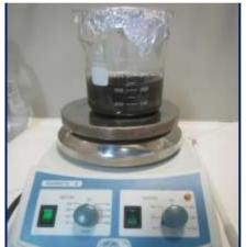
Figure 6. Sand sample shaking for 20 minutes
