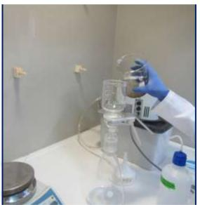
Figure 9. Filtration system with a 10µm polycarbonate filters.
