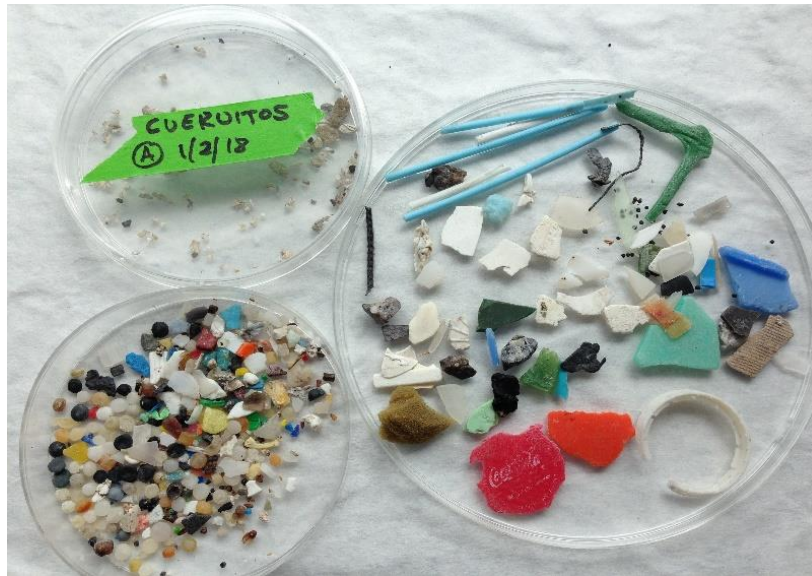
Fig. 9. Photograph of the sample 1-25 mm collected at Cuervitos beach on 1/2/2018. On the left, the larger microplastic (1-5 mm), and on the right the fraction of mesoplastic (5-25 mm).
