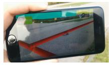
Figure 2, Underground infrastructure stored as CityGML visualised as AR on-site.
