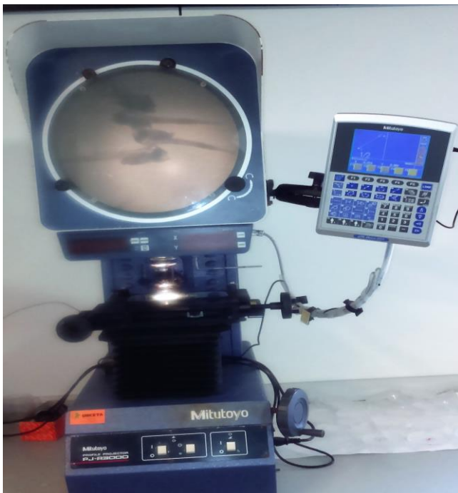
Figure 4. The PJ-R3000 profile projector. It used to measure larval length.
