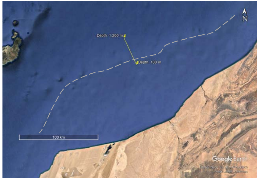
Figure 12. Google Earth® image showing the continental slope (dashed line). The depth changes 1,100 m in about 36.5 km (from Google Earth).
