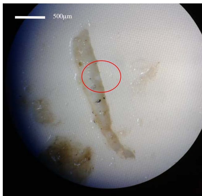
Fig. 18. Hot needle test on a white MP fragment
