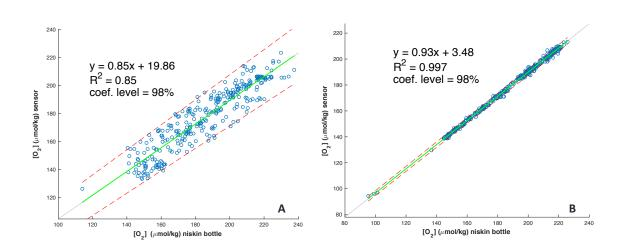
Figure 3. Comparison of dissolved oxygen concentration data of niskin bottles versus continuous data provided by the SBE43 dissolved oxygen sensor for Leg3 (A) and Leg5 (B) oceanographic cruises. Straight green line refers to the regression line. Red discontinuous line shows the confidence level for each oceanographic cruises at 98%. In both graphs the respective regression line equation and R<sup>2</sup> is shown.
