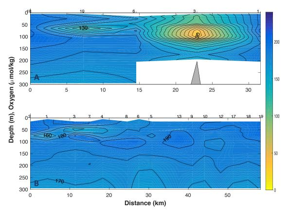
Figure 6. Vertical contours of dissolved oxygen concentration versus distance from specific transects of Leg3 (A) and Leg5 (B).
