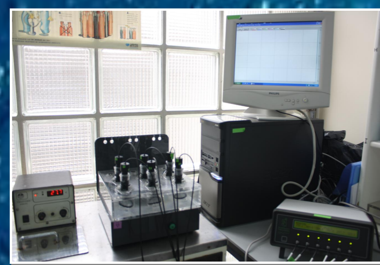
Figure 3. At the end of each period of starvation five individuals were separated for measurements of in vivo respiration (µl O 2 per hour) with oxymeter (Strathkelvin 928 6-Channel oxygen system) in individual cells of 50 ml at 20.5°C in dark conditions.
